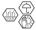
Dry to touch 1 hour, dry to use for light duty service 2 days (48 hours) for rough service allow 7 days (1 Week). Do not expose the truck bed to direct sunlight or rain for 8 hours after application.
